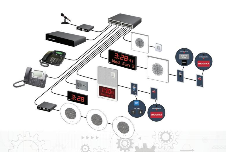
For facilities with existing analog technology, a hybrid approach is available allowing existing hardware and cabling to be re-used with the upgraded ethernet-based head end. This provides advanced mass notification coverage, increased speaker/display coverage, etc. and is an economical approach to the transition.
