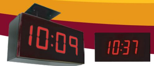
Telecor's IP PoE Clocks keep time accurately without the need for a Master Clock to provide synchronization. Time is set by Simple Network Time Protocol (SNTP). These clocks connect directly to a standard Ethernet jack drawing time updates from the network. Power to the clock is provided by Power over Ethernet (PoE) that delivers DC power to Ethernet-connected devices.
