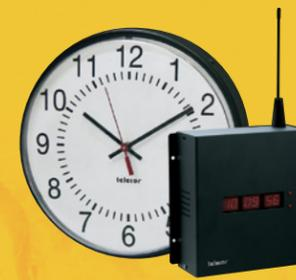
Telecor wireless analog clocks each receive and transmit a correction signal thus creating a wireless network of secondary clocks. The correction signal is relayed from the Telecor Master Clock to the Telecor Transceiver, which in turn transmits the signal to the clocks. Because each wireless clock in network functions as a receiver/transmitter, clock locations throughout a facility are not limited to the distance or signal path between the Transceiver and clocks.
