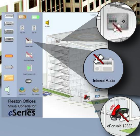
eVisual Console integrates with eSeries Fault Monitoring. In the event of a field device fault, trouble tones sound and the appearance of trouble icons draw attention to the fault condition. eSeries devices are monitored for network connectivity, line faults, and operability.
